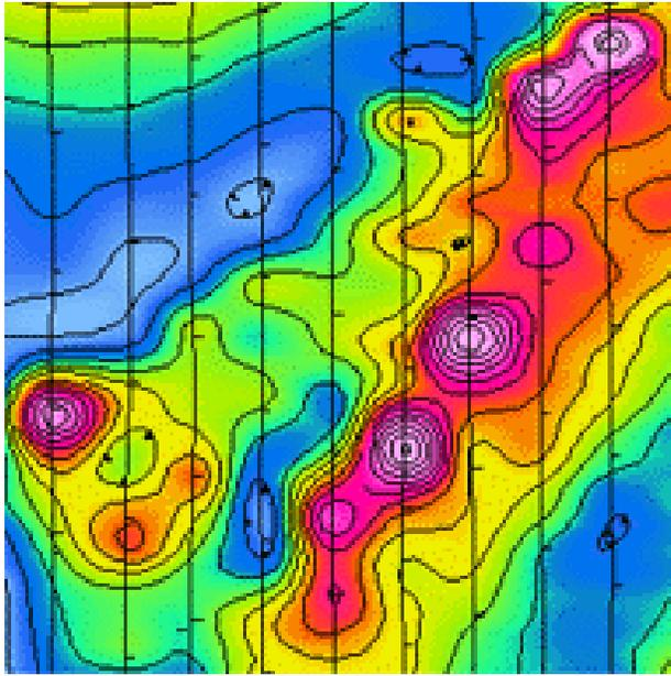
Figure 3. This magnetic map is looking at the ground as if from an airplane. The circular magnetic highs represent the kimberlite pipe. This is the diamond bearing pipe that goes deep into the ground.
