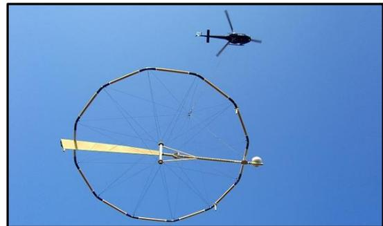
Figure 1. Helicopter performing an airborne electromagnetic survey.
