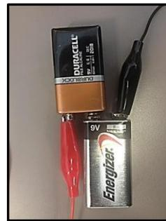
Figure 7. Two 9 V batteries connected in series.
